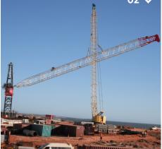
AUGUST 2010 – SEPTEMBER 2015 (Barrow Island): Working with KJVG, Marr's team erected a Favelle Favco M2480D tower crane to unload freight at the MOF at Wapet Landing on Barrow Island. The solution reduced barge unloading and repacking times from 4-5 days to a day.
